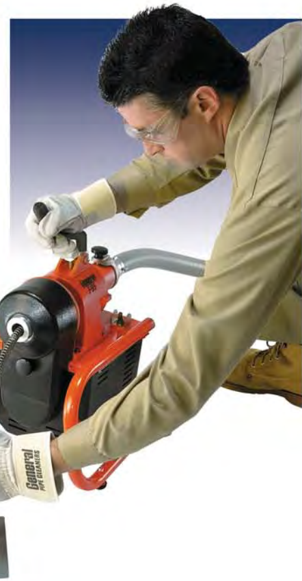
Clear 2" – 3" lines up to 125 feet long with 5/8" x 7-1/2' sections or 4" lines up to 150 feet long with 7/8" x 15' sections.
